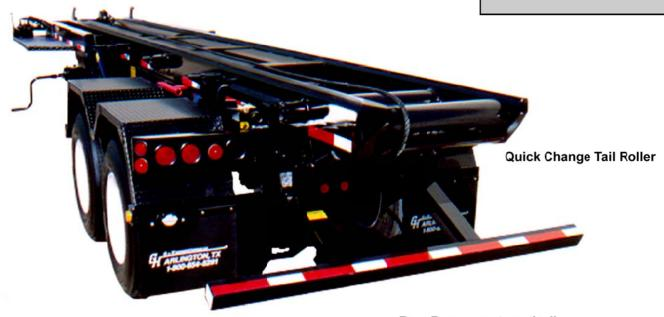
Rear Bumper automatically folds as the Hoist is raised
